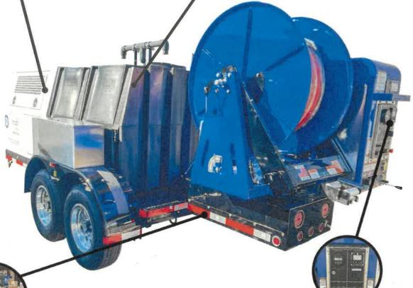
BOX TUBE FRAME: A steel box tube cross section is stronger than a "C" channel cross section and also leads to a stronger and longer lasting frame designed to withstand the strenuous rigors of any application you throw at it. It is for this reason we utilize this concept in all our products and provide our customers with the best value in the market.
