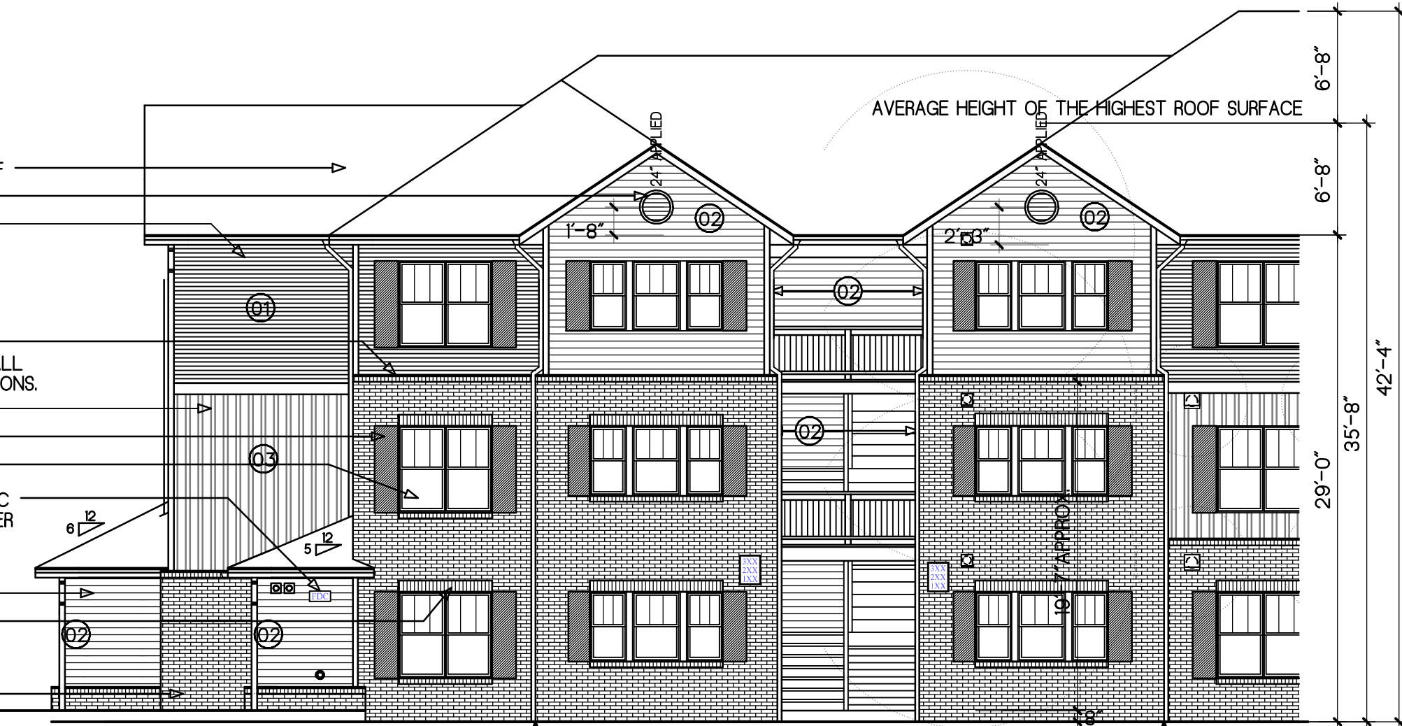
TYPICAL FRONT ELEVATION (3223-3 SHOWN) SCALE: 1/8" = 1'-0" (24X36)
