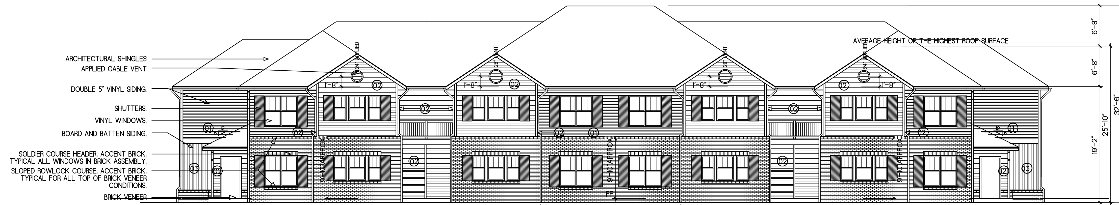
01 BUILDING TYPE 3223-2 FRONT ELEVATION A5.03 SCALE: 1/8" = 1'-0" (24X36)
